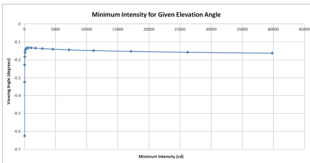
Figure 38 Minimum Intensities at Viewing Angles. Source 30 m high, observer 10 m high
